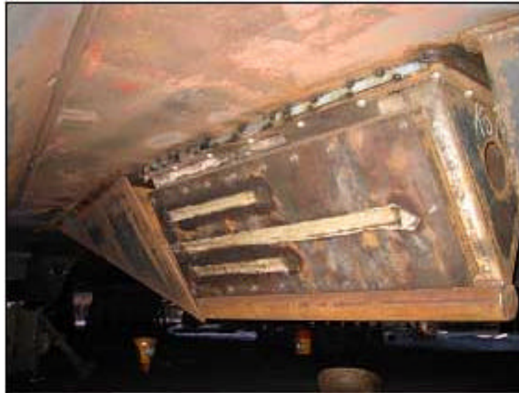
Figure 1: Sonar antenna on the bottom of the ice-"Kola" ship in the Arctic Ocean mission of 2003 devoted to the studies of bottom conditions for optical cable cabining (PolarNet project)
